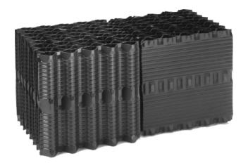
Modules are fabricated in 12", 24" and 48" depths, 12" to 24" widths, and in lengths up to 10'-0" in 2' increments. Custom dimension modules are available upon request. Standard sheet mil thickness is 15 mil after forming.
